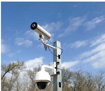
IVC FV-3532-01 deployed with legacy PTZ camera.
