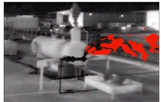
The FV-3532-01's thermal hydrocarbon leak detection camera under test at the TEEEX Training Center. Propane under pressure is being detected by the camera.
