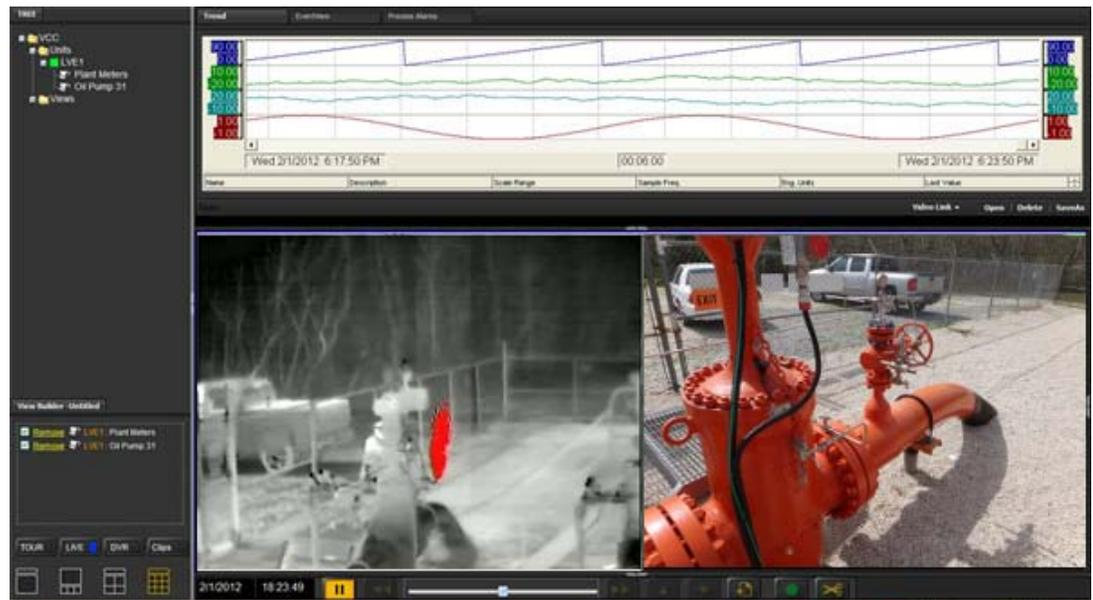
IVC's Longwatch Video System is used to treat video from remotely deployed cameras as additional process data. The Longwatch Video Historian can then correlate saved video clips from the site with other process data from the SCADA historical database to provide a more accurate picture of what is happening at the site
