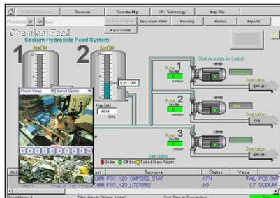
IVC's video management software is fully compatible with ActiveX, allowing seamless video integration into SCADA systems and other HMIs.
