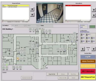
Operators view and control the system using touch screen monitors that simplify operation thereby significantly reducing training costs. IVC View Station Software is configured for the touch screens with buttons assigned and intuitively labeled for each of the various operations.
