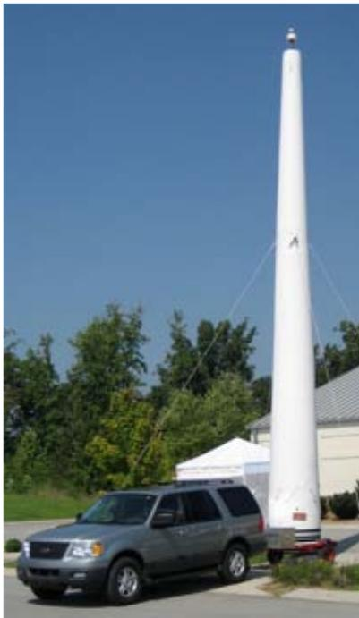
The towers come equipped with an IR sensitive 36x optical zoom camera and a long ranged IR illuminator to allow for clear images in low-light conditions.
